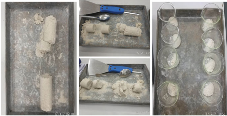
Fig. 6. Photographs of the treated sand columns and the sectional samples used for the carbonate content measurement by dissolving method
