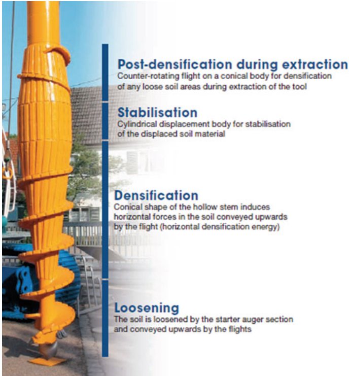
Fig. 2. An displacement drilling tool
